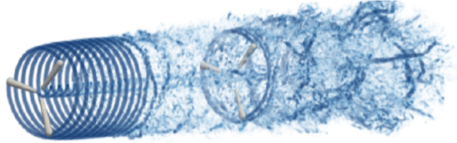
Wind field approximation & Turbulent flow around the wind turbine
